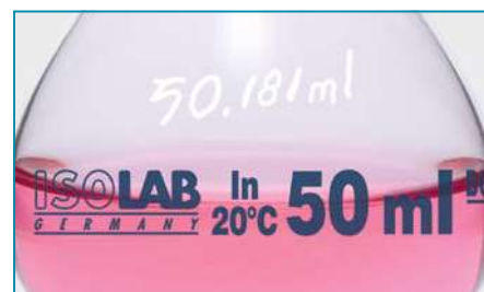
Net volume with 0,001 ml precision is engraved on the body of calibrated density bottles.
